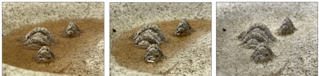
<Figure 6> Surface Changes through Pooling, Absorption, and Drying after Pouring
